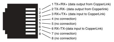
Figure 7. CopperLink Ethernet Extender 10/100Base-T RJ-45 Connector Pinout.
